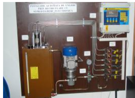
Figure 19: The recirculation lubrication system with electronic monitoring
