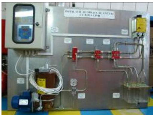
Figure 18: The lubrication systems with two lines
