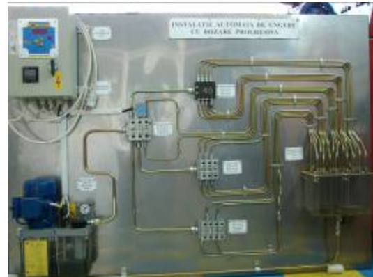
Figure 17: The progressive dosing lubrication systems
