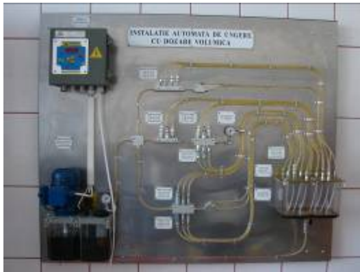
Figure 16: The volumic dosing lubrication systems,
