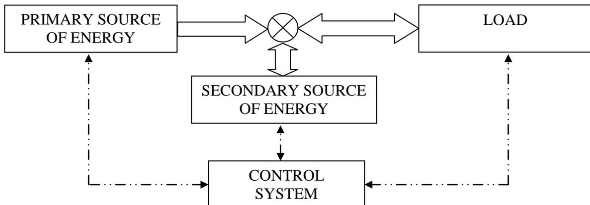
Fig. 2. Schema of parallel hybrid drive system [4].
