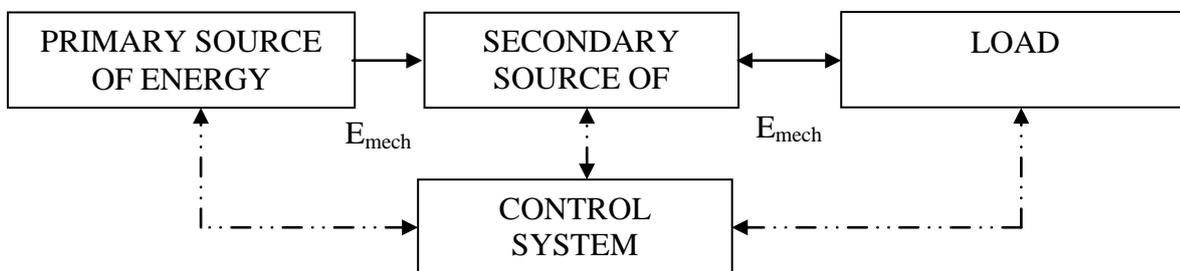
Fig. 1. Schema of series hybrid drive system.
