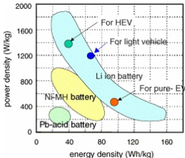
Fig. 5. Comparison of energy densities of rechargeable batteries [18].
