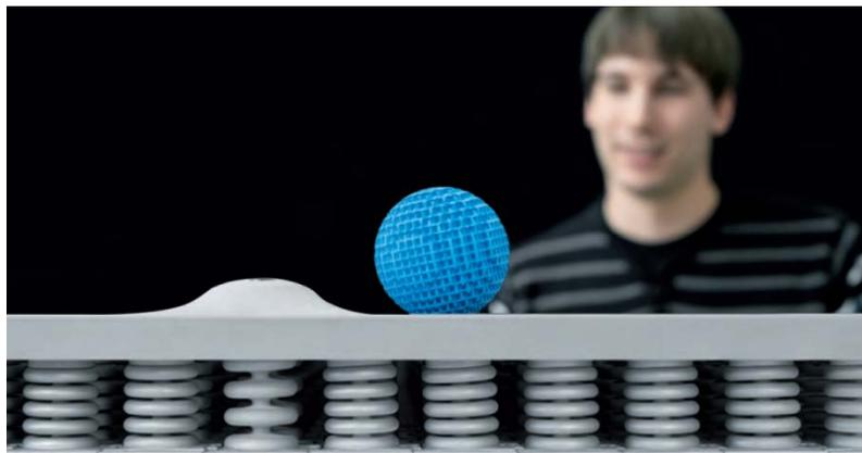
Fig. 5 The way the pneumatic cylinder operates on the conveyor membrane
