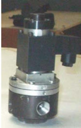
Fig. 7 Proportional pneumatic pressure regulator with membrane
