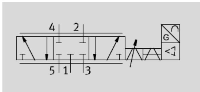
Fig. 2 Schematic diagram of operation of pneumatic directional control valve type MPYE from FESTO.
