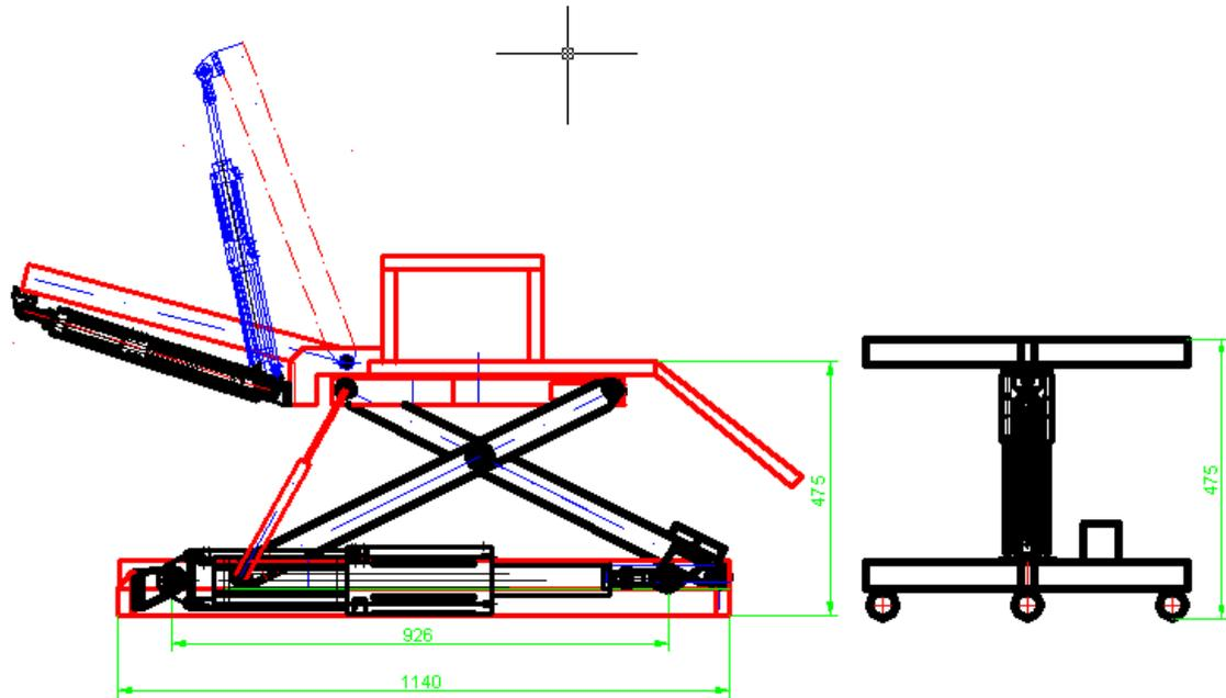
Fig. 9 Dental chair and small table operated by proportional equipment
