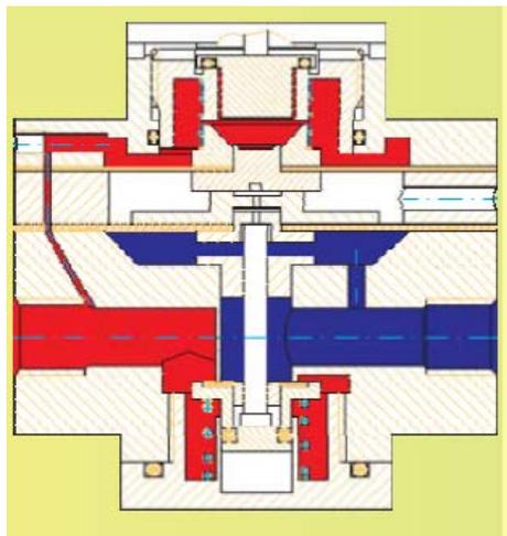
Fig. 8 Section through proportional pneumatic pressure regulator with membrane
