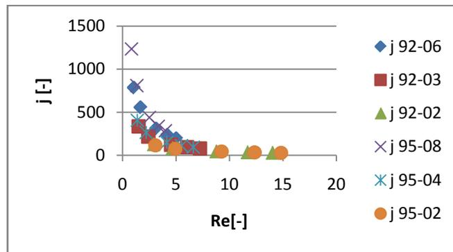
Fig. 5. Colburn factor plotted against permeability-based Reynolds number
