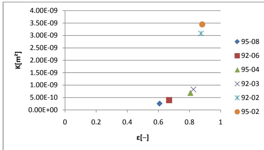
Fig. 9. The permeability of compressed foams is plotted against the values of measured porosity.
