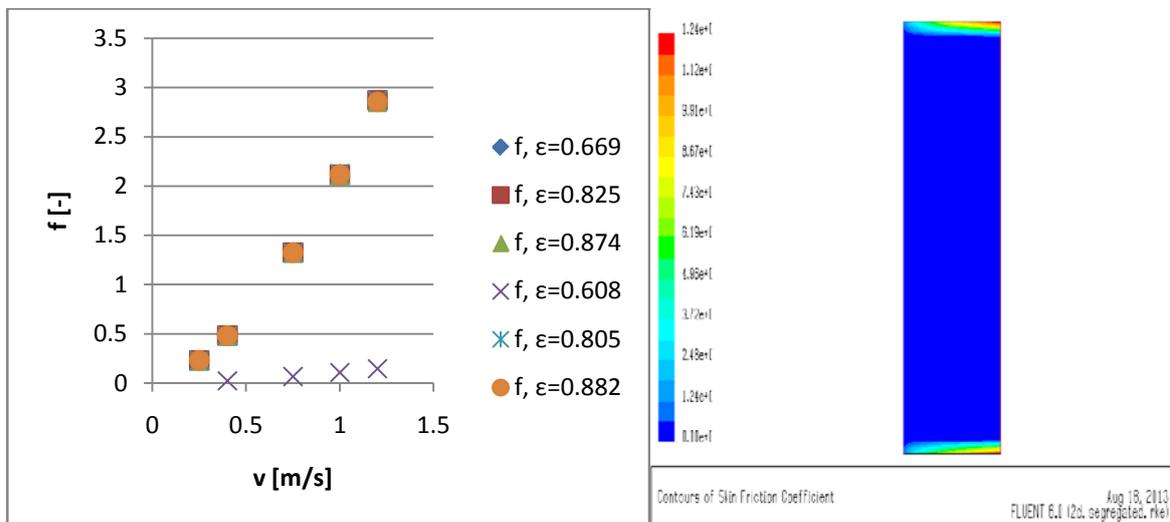
Fig. 8. Friction factor plotted against darcian velocity and contours of skin friction coefficient.
