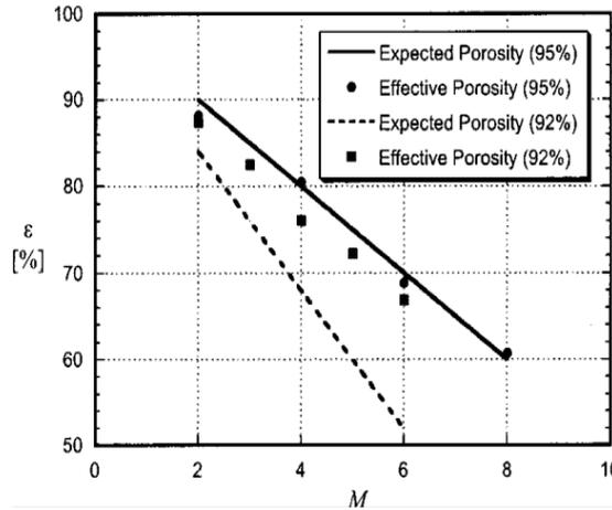
Fig. 1. The expected compressed metal foams porosities based on the precompression porosity and nominal compression factor compared against measured values [1].
