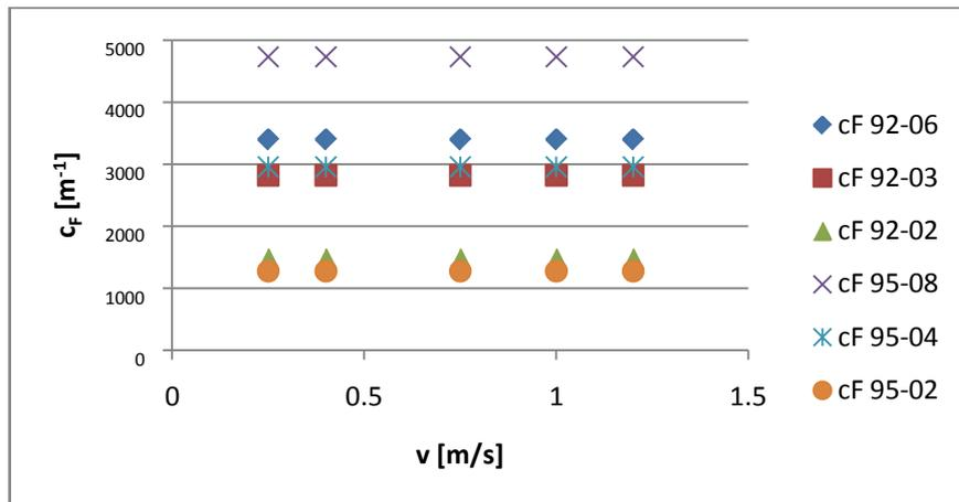
Fig. 10. The form coefficient of compressed foams is plotted against the darcian velocity.
