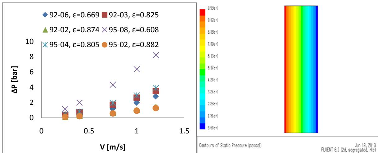
Fig. 7. Pressure drop versus fluid velocity for compressed foams and contours of static pressure.
