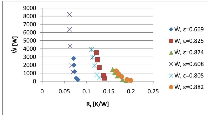
Fig. 6. Plot of the required pumping power against the corresponding thermal resistance.
