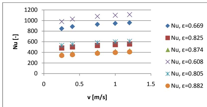
Fig. 4. Nusselt number plotted against flow velocity.
