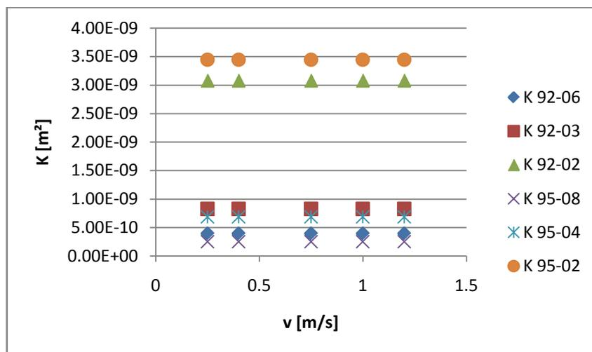
Fig. 11. Permeability plotted against darcian velocity
