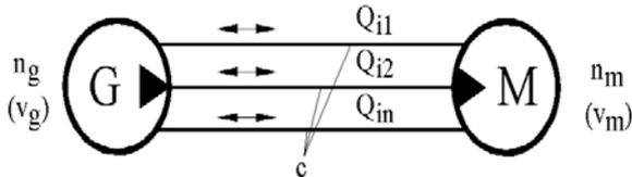
G-generator (pump), c-pipes, M-motor,  $Q_{ii}$  – instantaneous flow for phases i
