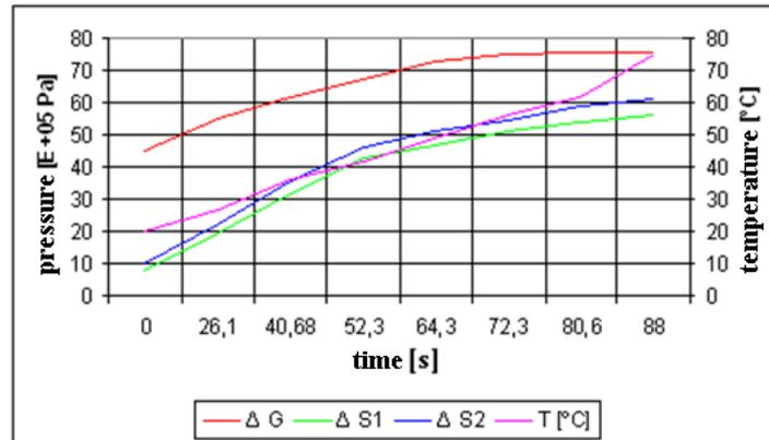
Fig. 3 Diagram of pressures and temperature variation with time in static pressure of 0,25E+05 Pa
