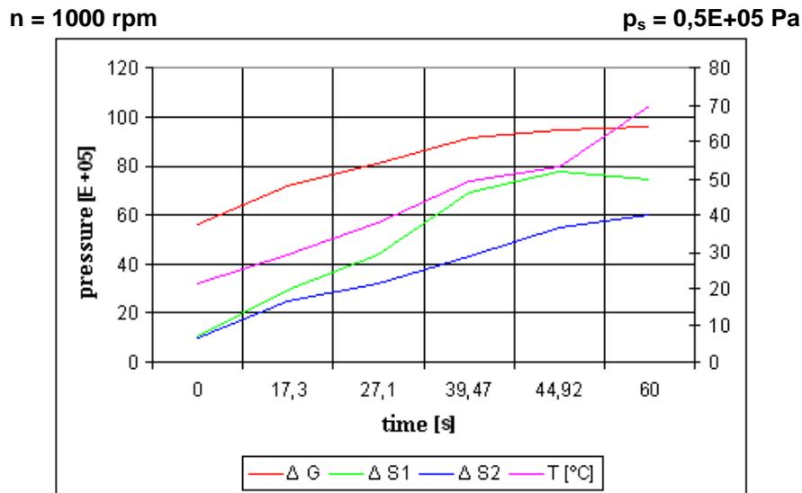
Fig.5 Diagram of pressures and temperature variation with time in static pressure of 0,5E+05 Pa
