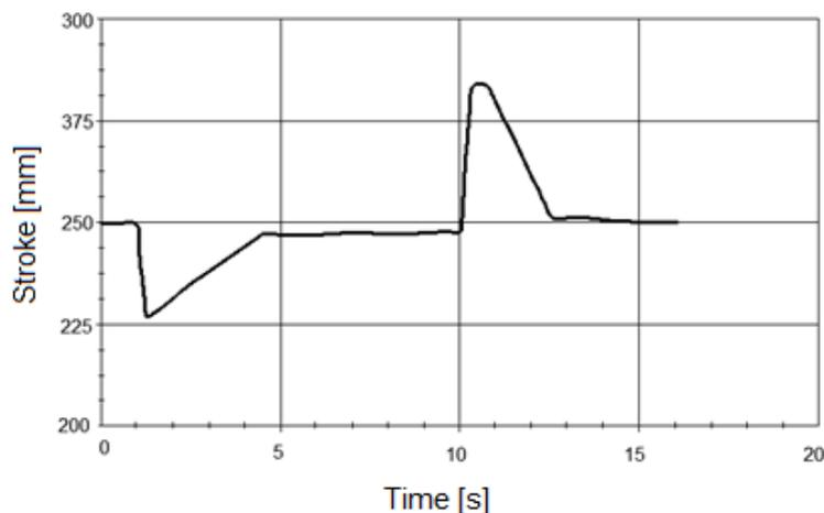
Figure 4 – Stroke diagram of the pneumatic actuator (9).
