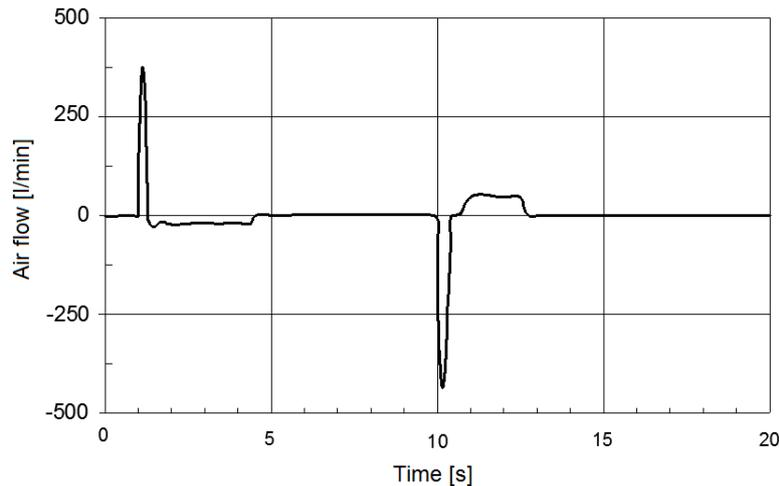
Figure 5 – Air flow variation diagram in the pneumatic actuator (9).
