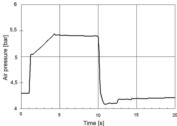
Figure 6 – Air pressure variation diagram in the pneumatic actuator (9).
