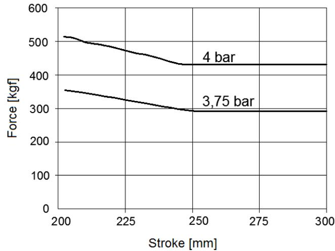
Figure 1 - Characteristic diagram of the pneumatic spring.
