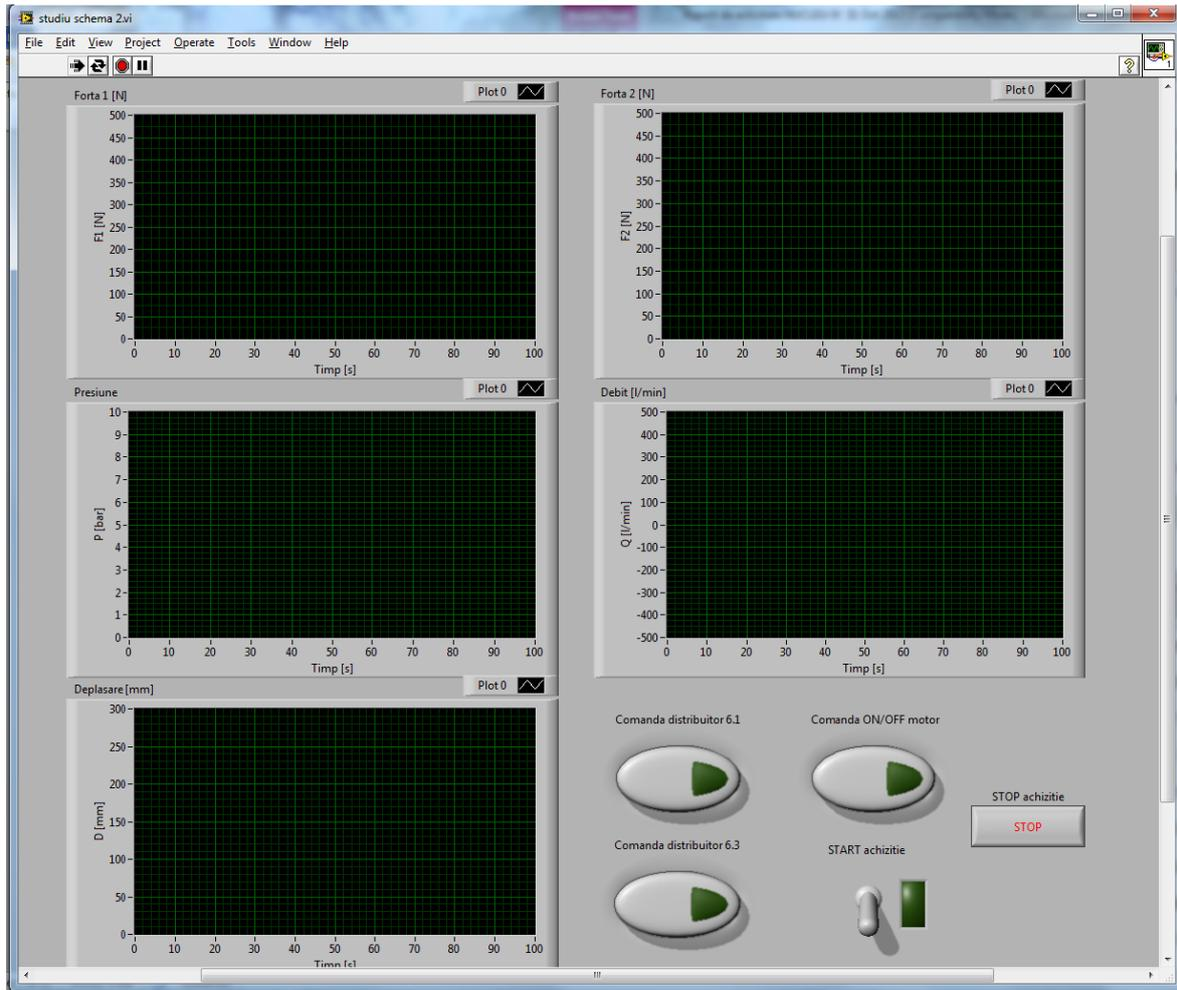
Figure 3 – Data acquisition and control virtual instrument.
