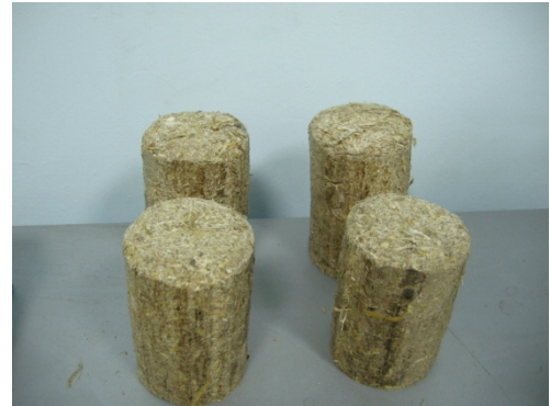
Fig.11 Maize stalks briquettes obtained on the sawdust presses
