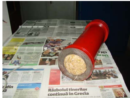
Fig.8 Briquette in the pressing cylinder; it is shown how the material is compacted
