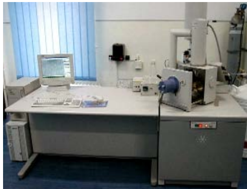
Fig. 1. Overview of electron microscope. XL-30-ESEM TMP.
