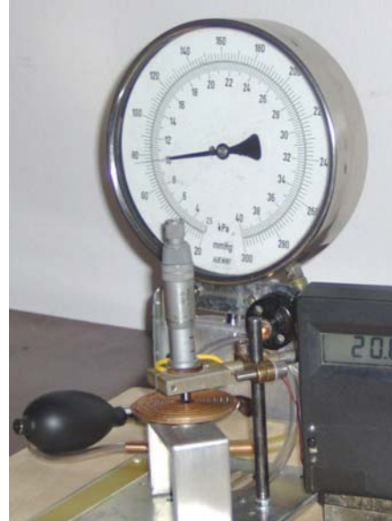
Fig. 1. MCDR-MM-01 - The equipment for measuring the deformations of corrugated capsules, when into these capsules are applied low pressures
