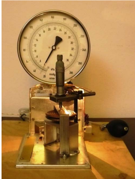
Fig. 1. MCDR-MM-01 - The equipment for measuring the deformations of corrugated capsules, when into these capsules are applied low pressures
