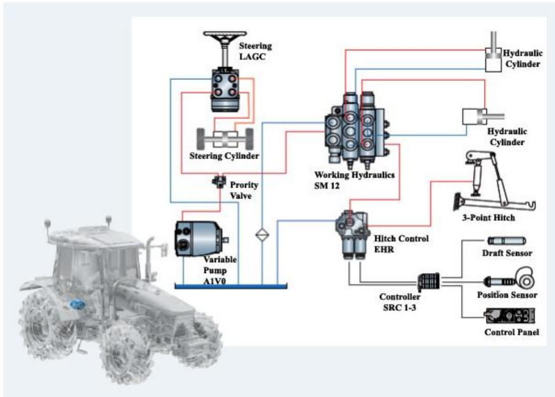
Fig. 1. Block diagram of a 90 HP agricultural tractor, [4]
