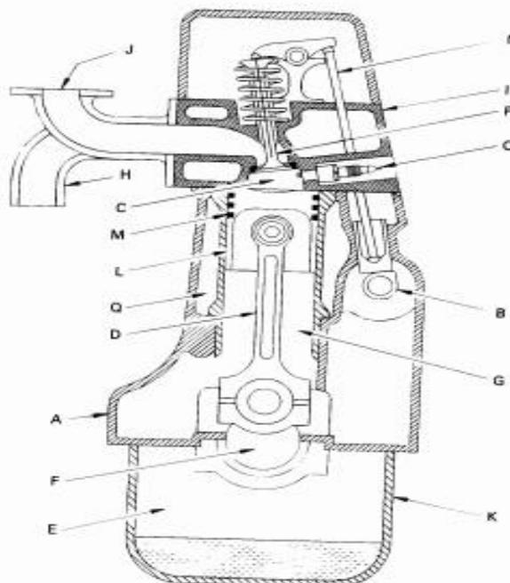
**Fig. 6.** Parts of Engine – Cross section of four-stroke cycle SI engine showing engine components; (A) block, (B) camshaft, (C) combustion chamber, (D) connecting rod, (E) crankcase, (F) crankshaft, (G) cylinder, (H) exhaust manifold, (I) head, (J) intake manifold, (K) oil pan, (L) piston, (M) piston rings, (N) push rod, (O) spark plug, (P) valve, (Q) water jacket.
