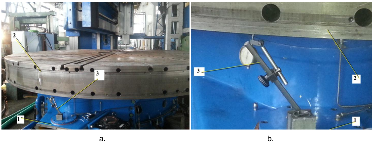
Fig. 16. Adjusting and checking the thickness of the oil film
