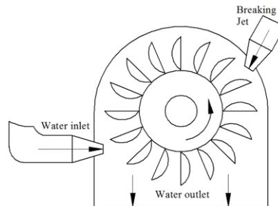
Fig. 1. Schematically representation of PELTON turbine
