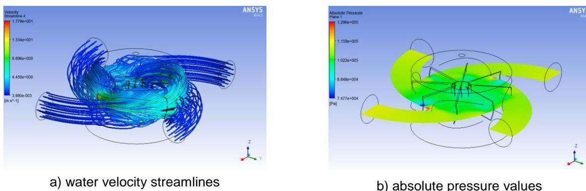
Fig. 5. The result obtained from the flow analysis
