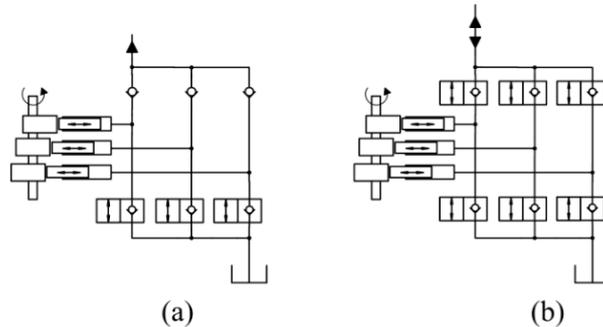
Fig. 5. (a) Piston type digital pump; (b) pump-motor [1]
