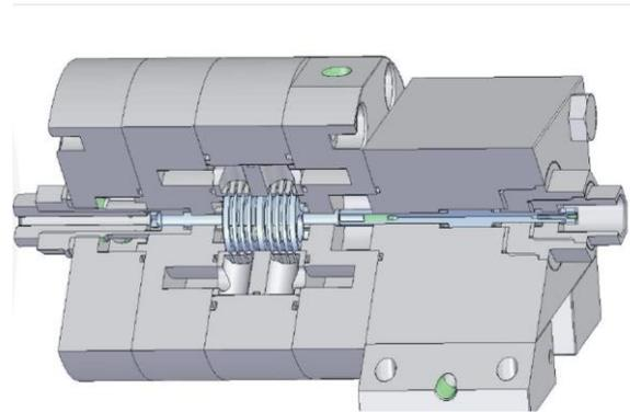
**Fig. 7.** CAD model of the fast switching linear valve [6]
