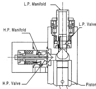
**Fig. 2.** Cylinder head arrangement of a digital-displacement pump-motor [2]
