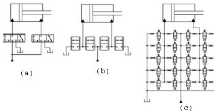
**Fig. 4.** (a) 2-three-way proportional valve distributed system; (b) 4- two-way valve system; (c) a digital on-off valve system [1]
