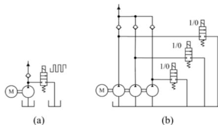
Fig. 1. (a) Switching pump; (b) parallel connected pumps [1]
