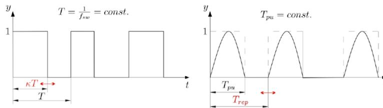
Fig. 6. PWM (left) and PFC (right) and their characteristic values [6]
