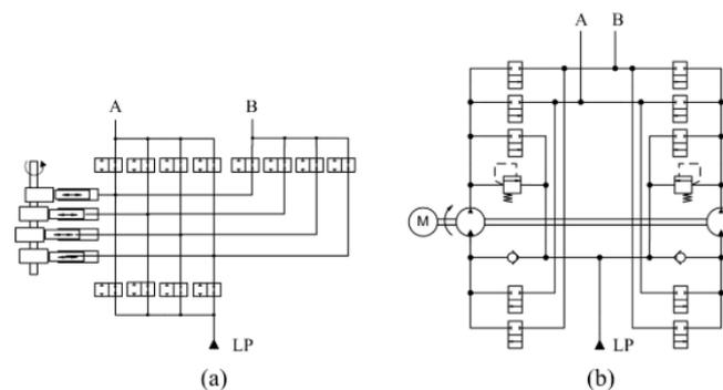
**Fig. 3.** (a) Two-outlet piston type DHPMS; (b) DHPMS based on fixed-displacement units [1]
