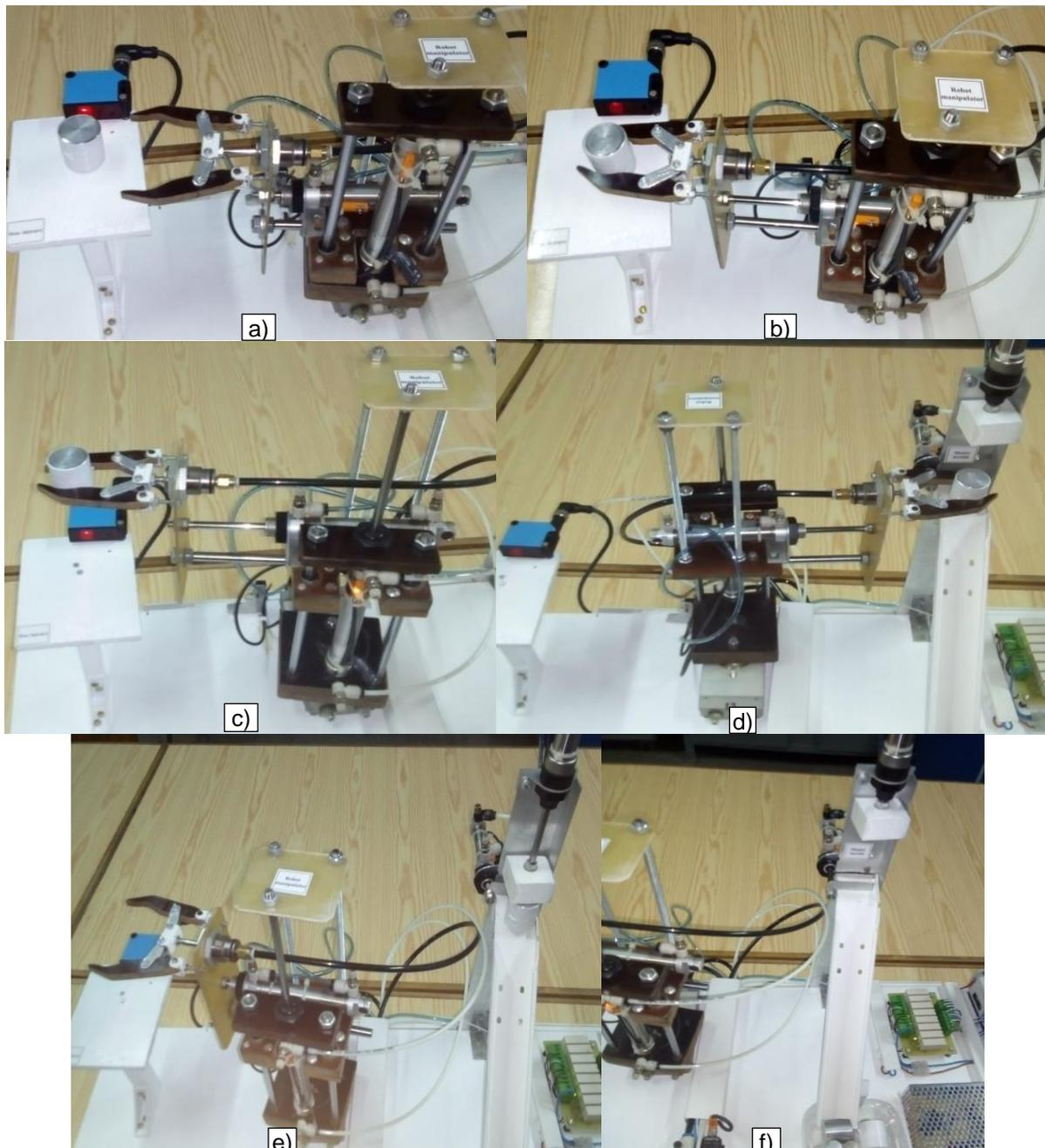
**Fig. 6.** Working states of processing station: a) piece detection; b) piece grip; c) lifting the piece; d) putting the piece on the tool machine; e) processing the piece; f) piece evacuation.
