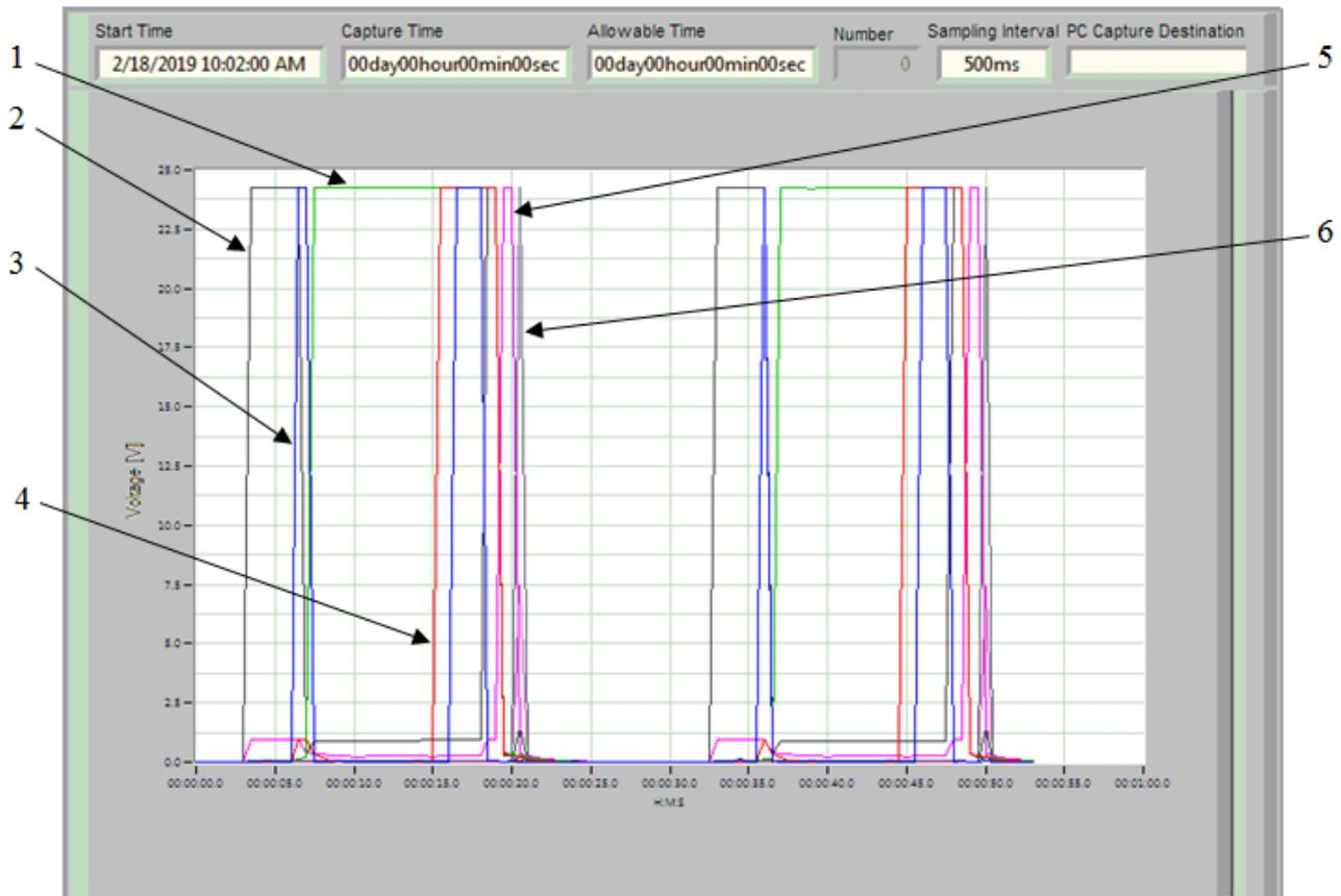
**Fig. 7.** Recording of command signal diagrams generated by PLC: 1- lifting arm of robot; 2- opening gripper; 3- robot arm pushing; 4- robot rotation; 5- piece processing; 6- piece evacuation.
