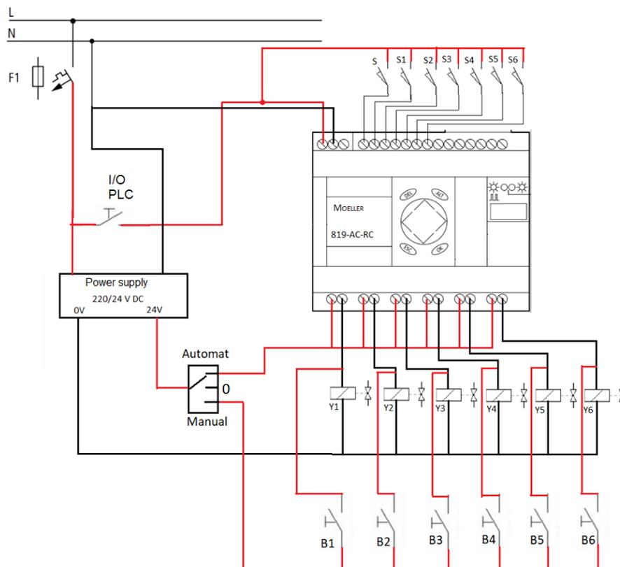
**Fig. 4.** Electrical circuit diagram of the processing station
