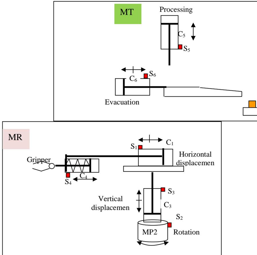
Fig. 2. Structure of pneumatic drive of the processing station
