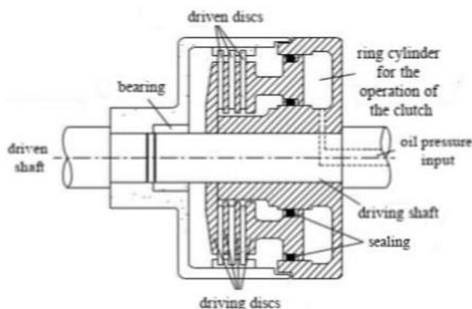
Fig. 1. The structure of a hydraulically actuated multidisc clutch [9]
