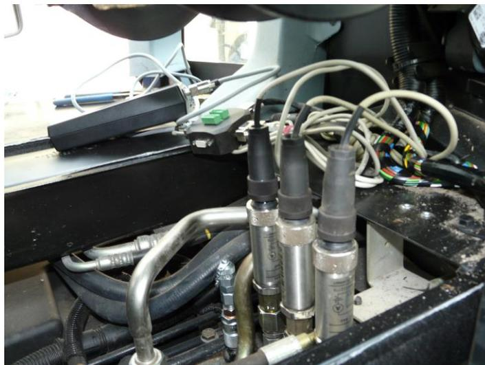
**Fig. 3.** Connection of the pressure transmitters and the data collector to the control block, valve C, D and E.
