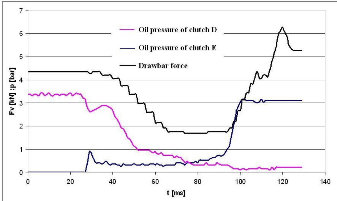
Fig. 6. Time course of the hydraulic control pressure and the drawbar force during gear shifting
