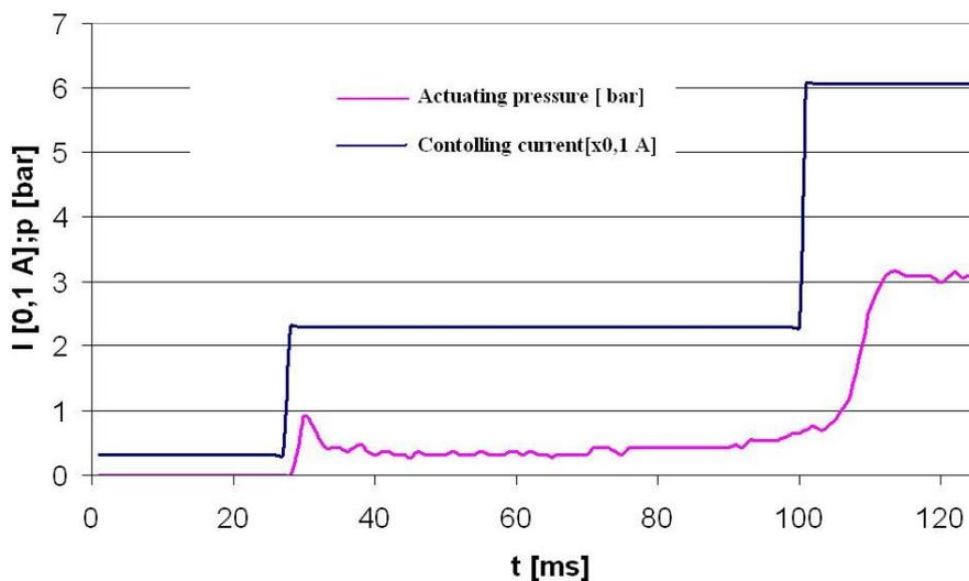
Fig. 5. Time course of the pressure of the electronic signal at clutch D and the hydraulic actuator during gear shifting
