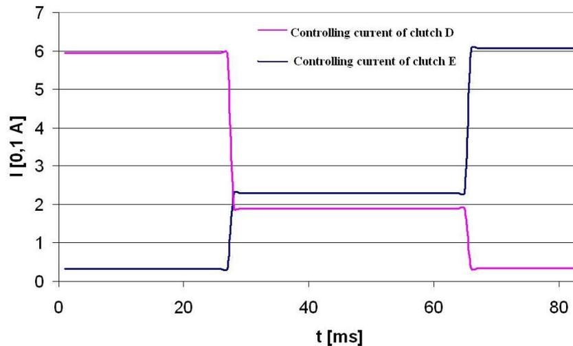
Fig. 4. Time course of the electrical control signals of the subsequent gears during gear shifting
