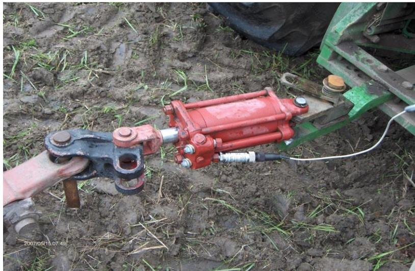
Fig. 2. Measurement of indirect drawbar force with hydraulic cylinder
