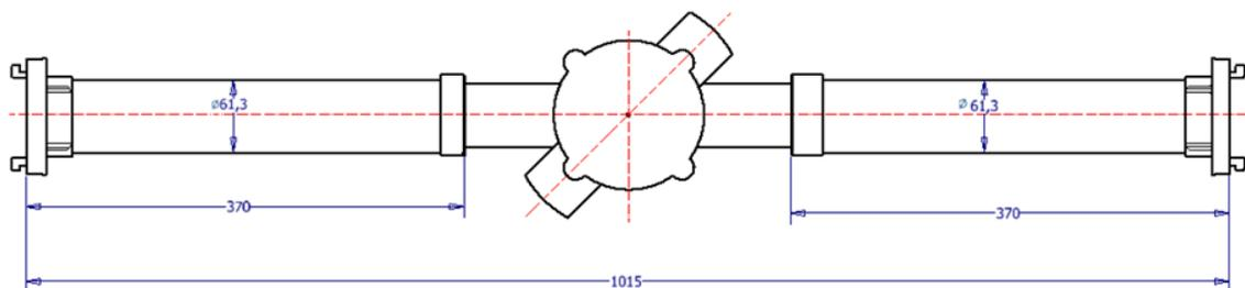
**Fig. 2.** Ultrasonic Flow Meter type Arad Octave 50 (Source: prepared by the Authors)
