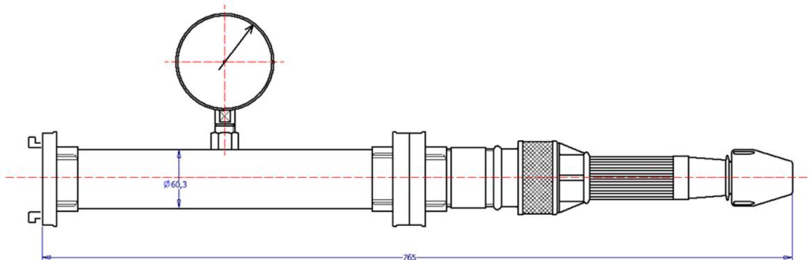
**Fig. 3.** The connected pressure gauge and measuring nozzle (Sources: prepared by the Authors)
