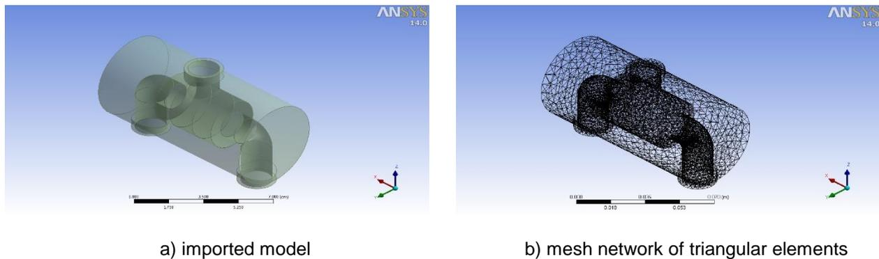
**Fig. 1.** Three-dimensional assembly model taken into consideration for flow analysis
