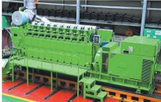
Fig. 4. Diesel main generator [2]
